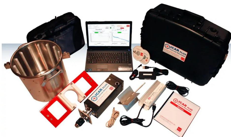
Rys. 5. Reometr ICAR Plus [8]
