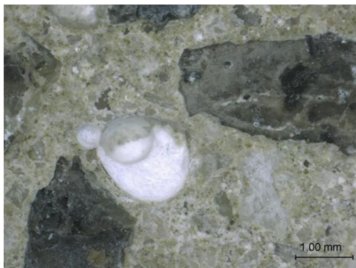
Fig.10: Light microscopic detail image of a saw-cut surface; surface concrete 0-8 without ASR-mitigating admixture
